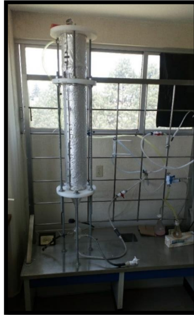
Figura 2.11. Reactor O 3 /UV
