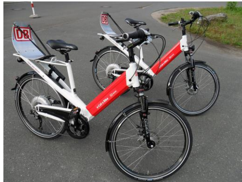
Figure 1.2. Riese und Müller "Jetstream". 3 Pedelec designed for the e-call a bike 4 service by the German railway (Deutsche Bahn) in Berlin
