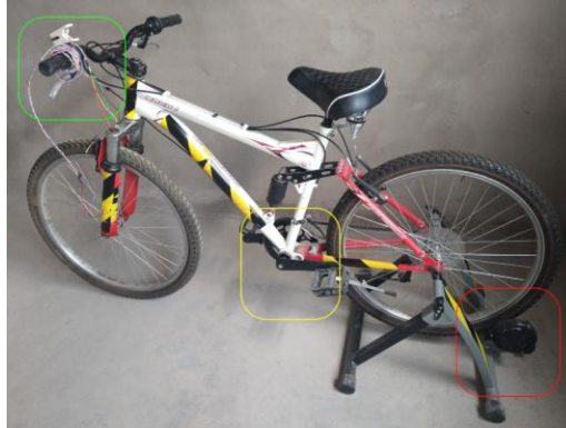
Figure 4.15. Test bicycle with the photoplethysmography sensor (green box) Torque sensor (yellow box) and magnetic resistance trainer (red box) to create different torque requirements.
