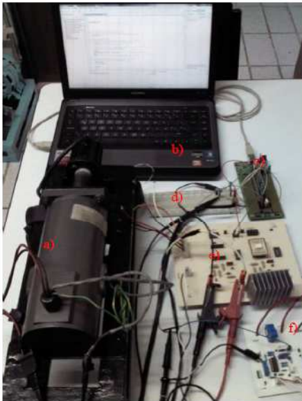
Fig. 6 Laboratory test prototype. a) PMDCM used, b) personal computer, c) digital platform, d) speed signal filter, e) power electronics, f) current sensor
