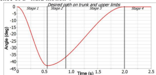
Fig. 5. Desired path for trunk and upper limbs on STS movement. A 42.9^\circ flexion is desired on 0.52s , which correspond to stage 1 of the movement. Remaining simulation time is used to return to anatomic position.
