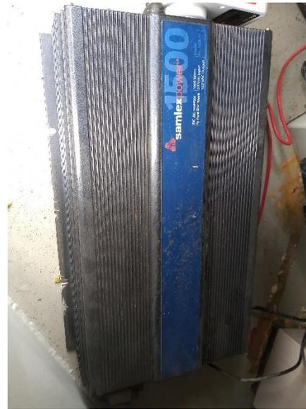
Fig. 23 Inversor de 1500w 24 VDC-120VAC.
