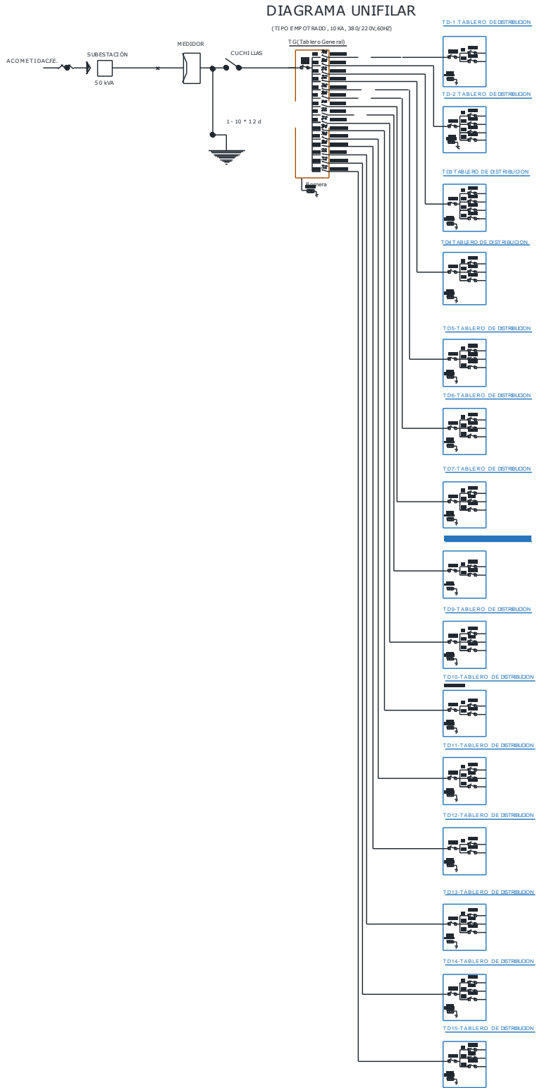
Plano 34: IE 10: Diagrama Unifilar
