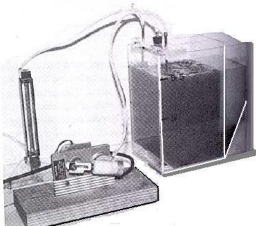
FIGURA 1 : REACTORES BIOLOGICOS, DE FLUJO CONTINUO Y POR LOTE (Tomados de Reynolds Tom: Units and Processes in Environmental Engineering.)
