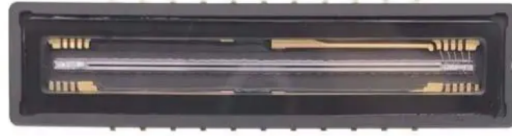
Figura 3.7: Sensor Toshiba TCD1304DG . Tomado de [32].
