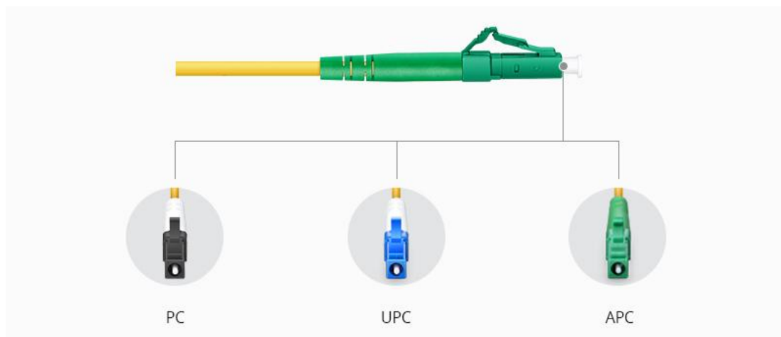
Figura 2.15: Conector PC vs. UPC vs. APC
