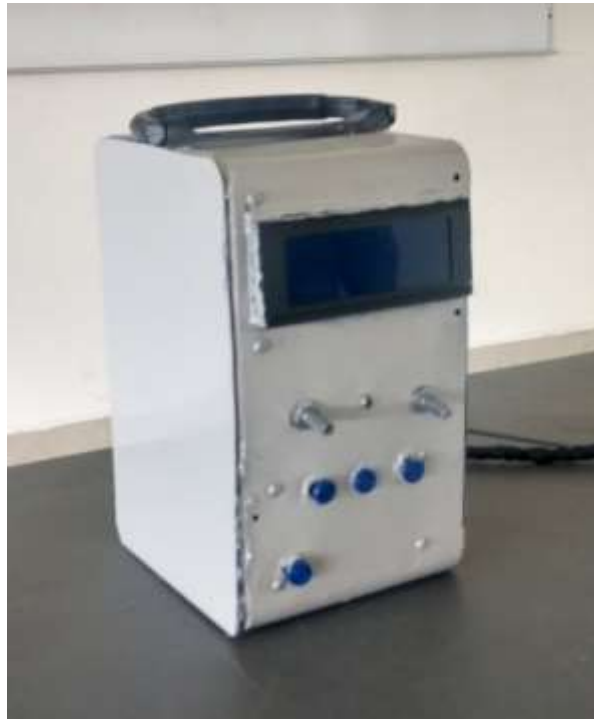
Figura 65. Caja panel de control (Gabinete).
