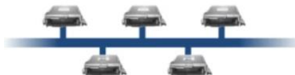
Imagen 2.29 Topología de red Bus. Tomada de FlexRay Automotive Communication Bus Overview , [fotografía], NI, https://www.ni.com/en/shop/seamlessly-connect-to-third-party-devices-and-supervisory-system/flexray-automotive-communication-bus-overview.html#section—1927873434
