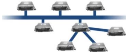
Imagen 2.31 Topología tipo híbrida. Tomada de FlexRay Automotive Communication Bus Overview , [fotografía], NI, https://www.ni.com/en/shop/seamlessly-connect-to-third-party-devices-and-supervisory-system/flexray-automotive-communication-bus-overview.html#section--1927873434
