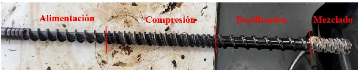
Figura 2.7. Husillo de extrusor Beutelspacher.
