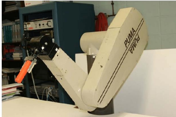
Ilustración 5 Robot PUMA 560, por Lin, Hsien-I & Lee, 2013, Measurement of the Robot Motor Capability of a Robot Motor System: A Fitts's-Law-Inspired Approach
