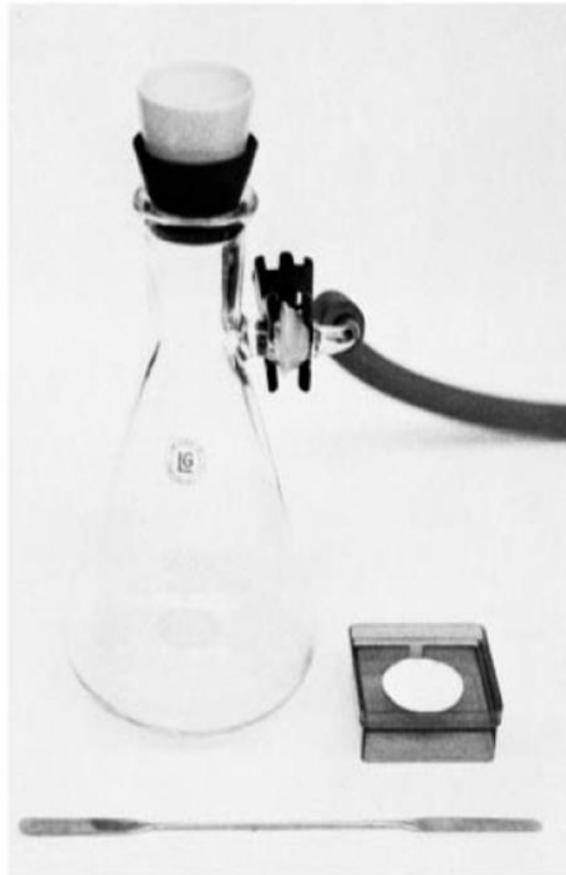
FIG. 2 Filtration Apparatus
