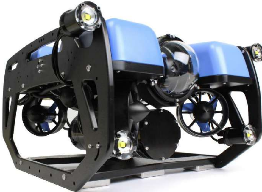
Figura 3.1- Robot submarino tipo BlueROV2 de BlueRobotics (BlueRobotics, s.f.).
