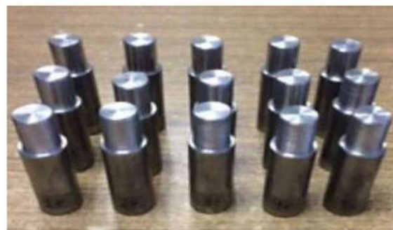
Figure 8 Machined shafts with different surface finishes (fine, medium and rough)
