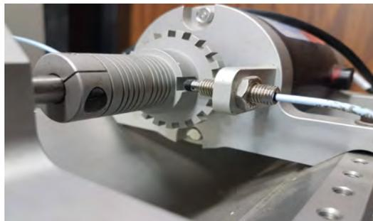
Figura 5.3: Tacómetro del banco experimental Bently Nevada RK4.
