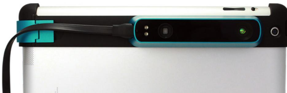
Figura 2.6: Structure Sensor.
