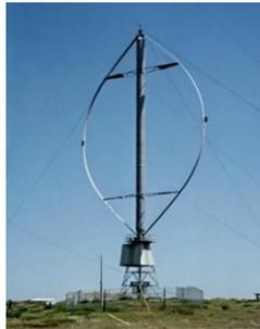
**Figura 2.6 Aerogenerador Darrieus (Aerogenerador Darrieus, 2019)**
