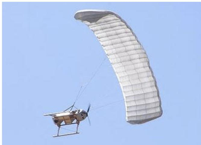
FIGURA 3. DRON DE ALA FLEXIBLE TIPO PARAPENTE.
