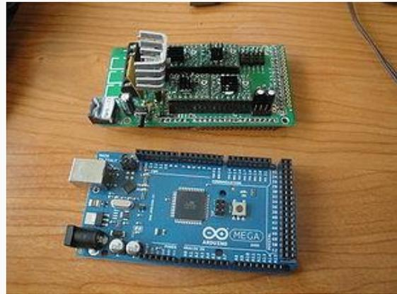
Figura 5. 2 Arduino Mega+RAMPS
