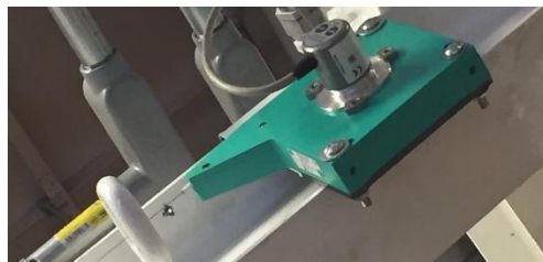
Figura 14. Encoder lineal ECA10TL-10ANP-I42BD.
