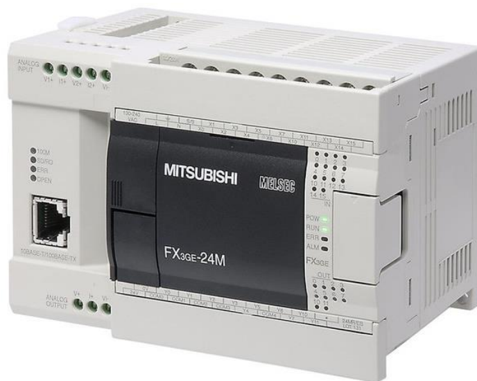
Figura 18. Figura III-PLC Mitsubishi FX3GE-24M.
