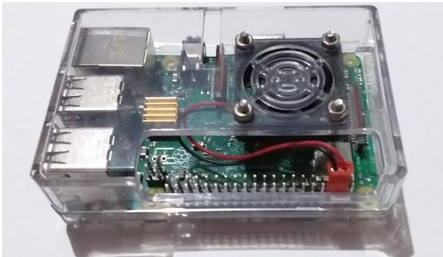
Figura 1.11 Raspberry Pi 3 Modelo B
