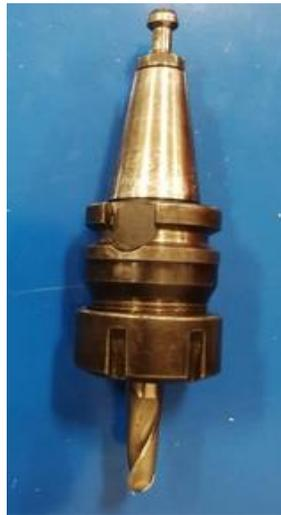
Figura 10. Fresa semicircular convexa 12.7 mm.
