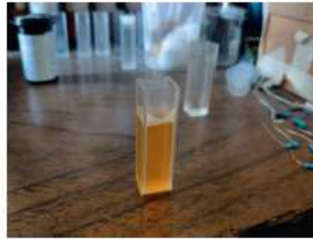
FIGURE 4: Blood plasma deposited in the quartz cuvette.
