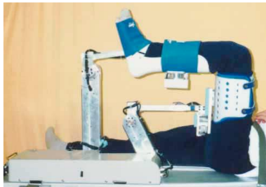
Figura 3.1. TEM: Therapeutic Exercise Machine (figura tomada de Sakaki, et al. 1999).
