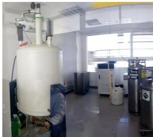
Figura 2.24 RMN Ascend <sup>TM</sup> 400 mHz y consola Avance 111 HD Marca Bruker.
