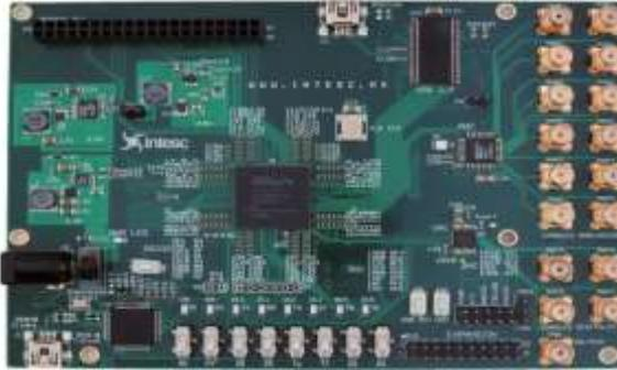
**Figura 2. 12: Tarjeta FPGA ASSERTA.**
