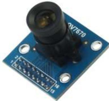
**Figura 2. 7: Cámara VGA OV7670.**
