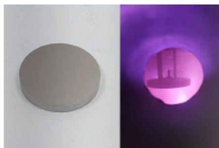
Figure 1 Mirror-polished 316L substrate. Plasma from the process of seed deposition by PVD
