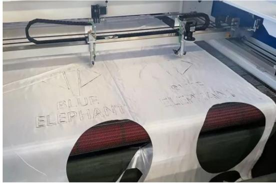
Figura 9 Double-head Automatic Feeding CO2 Laser Cutting Machine (Jack, 2022).
