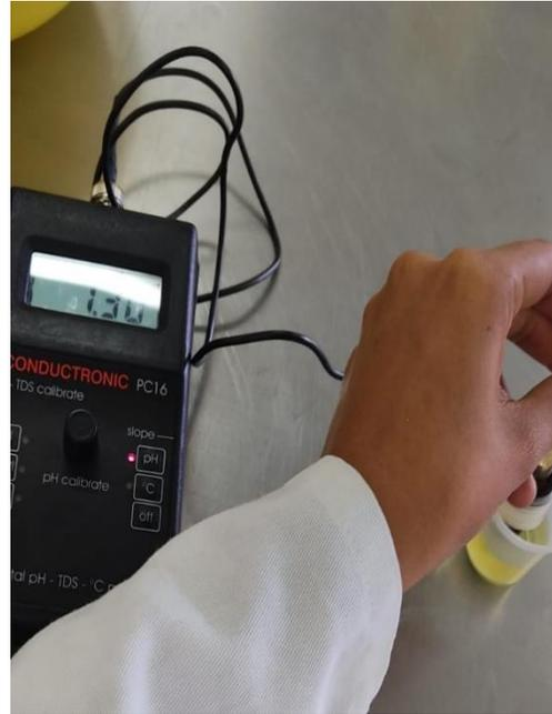
**Figura 61.** Calibrador de Buffer pH 7.0
