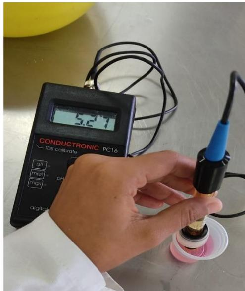
**Figura 60.** Calibrador de Buffer pH 4.0.
