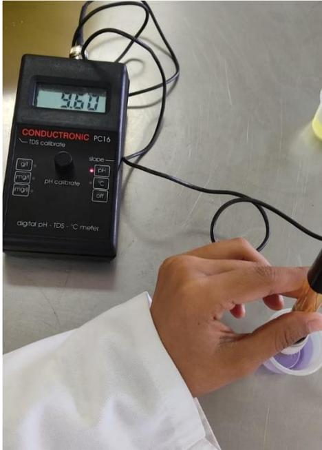
**Figura 61.** Calibrador de Buffer pH 10.0
