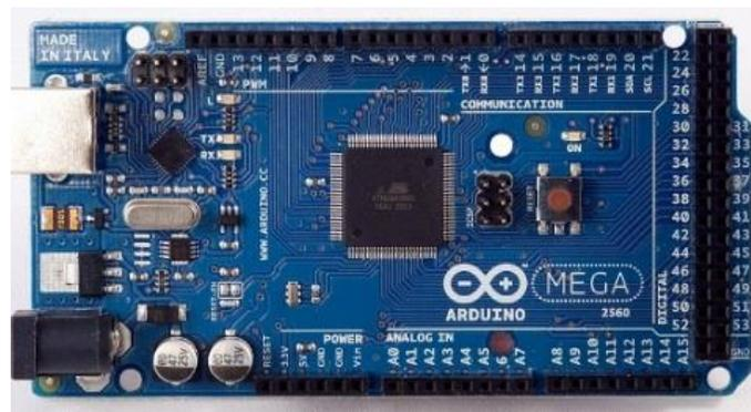
Figura 2.13. – Arduino Mega 2560.
