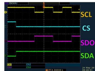
Fig. 15. Measurement of CS, SCL, SDO and SDA signals of the SPI in an oscilloscope.
