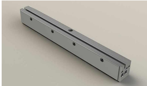
Figura 4. 25 Mordaza de sellado verticales ( Greener corporation, 2019 )
