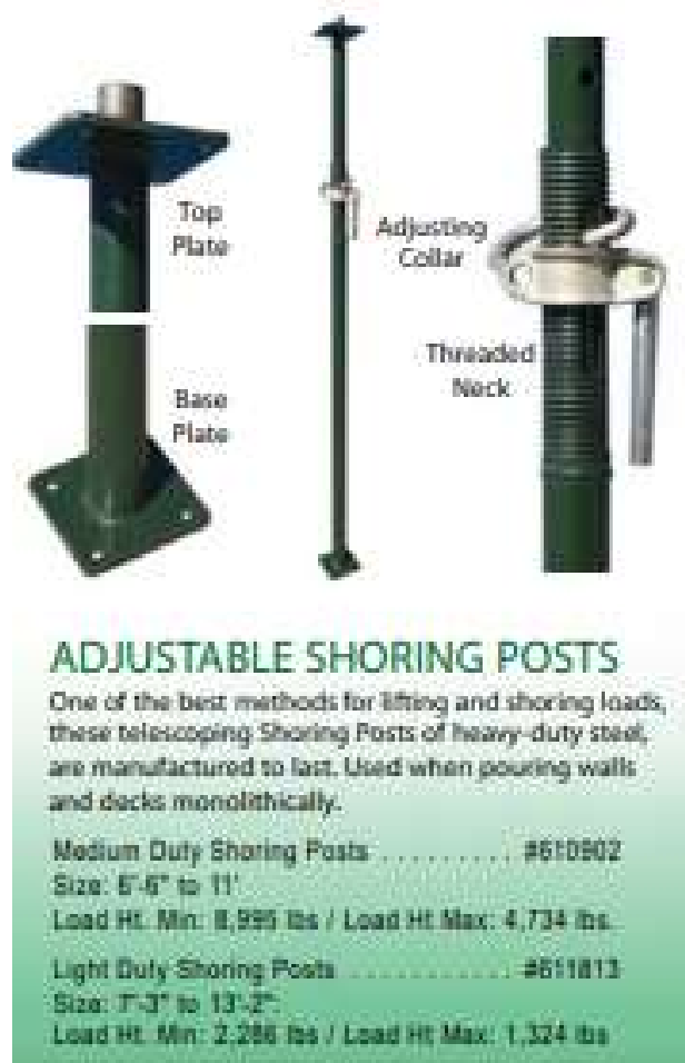
Figura 16. Postes para formaleta de losa. Fuente: https://8cc1a052-7ba2-410c-86d8-98c93d502599.filesusr.com/ugd/bca8bc_e2fa011fb092433eb1bd79798657b500.pdf
