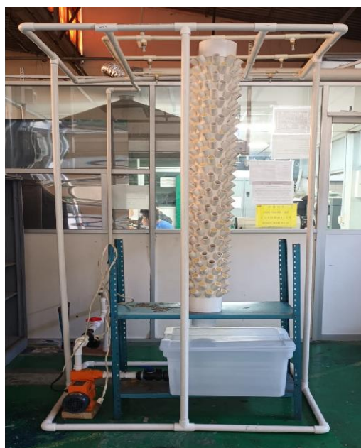
Figura 4.10 Ensamble general de invernadero vertical.
